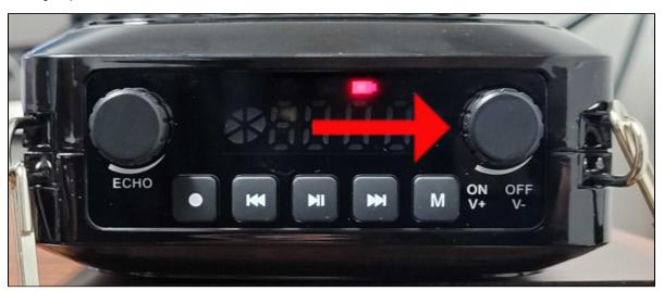
Turn on the microphone with the switch on the top of the microphone.
