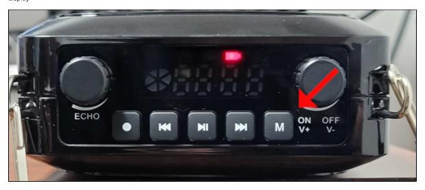
If you see "bt" or "line", you didn't hold the key long enough. Press the M key until "UHF" is displayed, then press and hold until you hear "UHF is waiting for connection".
